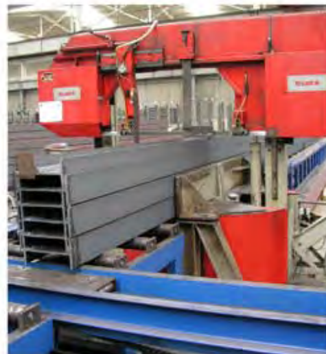
Cutting of rods and bars
