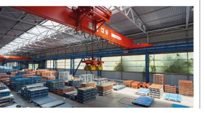
coils and single blocks are handled. The volume of manipulated metallurgical material handled by the 150 cranes in operation corresponds to about 2.3 million tonnes with about 1 million manipulations per year. The weight of the load suspended on the crane ranges from tens of kilograms to tens of tonnes.
